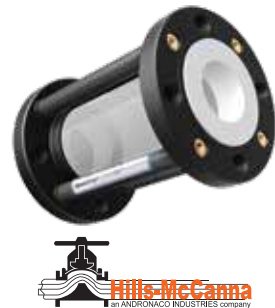
ChemTite® 360° Sight Flow Indicators: 1" - 12" up to 60" long Ductile housing and PFA lined for severe duty. Dovetail locking grooves for PFA retention. Pressure tested: 225 psig hydrostatic. Operating temperature (-)20°F to (+)350°F.
