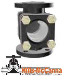
ChemTite® Bull's Eye Sight Flow Indicator: 1" - 6" Ductile housing and PFA lined for severe duty. Dovetail locking grooves for PFA retention. Pressure rating: 250 psi. Operating temperature (-)20°F to (+)400°F.
